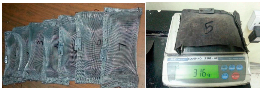
Figure 1. Deformable steel packages for feeding of Extruded Briquettes (brex) into Midrex reactor.
