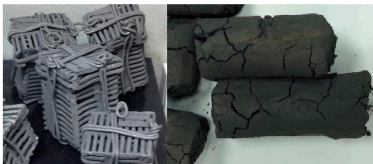
Figure 4. Rigid baskets for brex and the reduced cement-bonded brex after their extraction.
